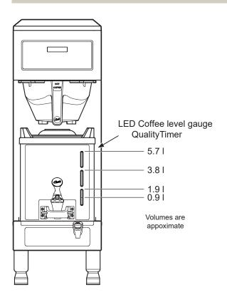
The LED coffee level gauge on the front of the satellite is also the indicator for the IntelliFresh Quality Timer system.
