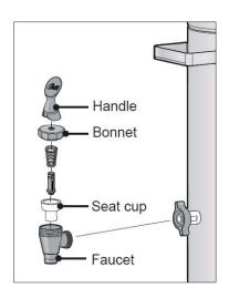
\* Reassemble - When dry, reassemble the handle/ bonnet. Hand tighten the handle/bonnet onto the top of the faucet assembly. Hand-tighten the faucet assembly onto the dispenser outlet.
